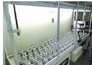
RIPPSS (RIKEN Plant Phenotyping System): this system controls individual soil moisture in continuously rotating 120 pots by a combination of automatic weighing and watering system, and monitors each plant size and expansion rate
