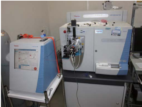
LC-MS system for peptide identification and quantification
