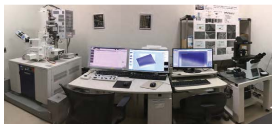
Fig4. MirrorCLEM system: FE-SEM equipped with a light microscope
