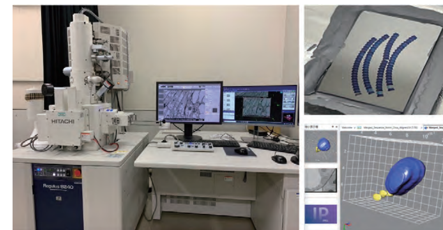
CLEM & array tomography system for electron microscope, serial sections and 3D image
