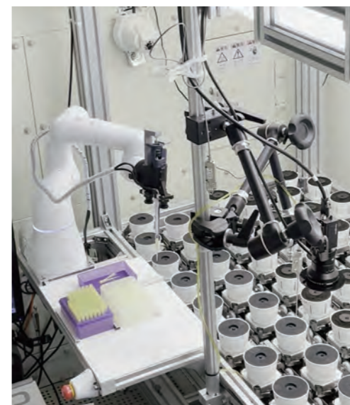
Automated chemical application system working with the plant phenotyping system RIPPS
